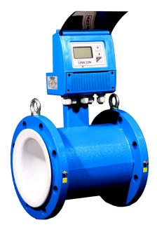
Faraday's Law states that a voltage will be induced in a conductor (the conductive fluid) when it passes through a magnetic field (generated by the meter), and that voltage will be directly proportional to the velocity of the conductor (the fluid). This voltage is measured by electrodes on opposite sides of the flow tube and used to calculate the flow velocity.
